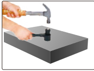
hammer impact to apply test force
